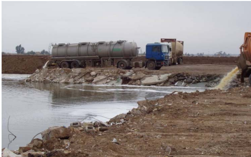
Figure B-9. Dumping of Wastewater in a Lagoon in Iraq Source: USACE, 2008
